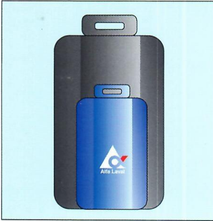
Fig. 4 SWPHE becomes more compact and request a lower filling of refrigerant for the same duty.
